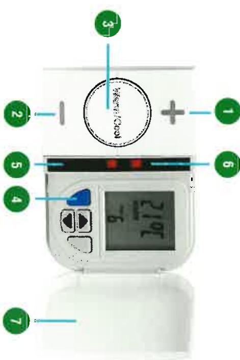
Warm is shown by red lights (6) and Cool is shown by a blue light (5). The centre button (3) marked 'Warm/Cool' allows you to toggle between warm and cool setting. When one or more red lights are on, you can increase the temperature by pressing the '+' button (1). For example, press once to go up by 1 degree C, or press twice to go up by 2 degrees C.
