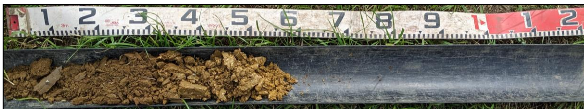
Photo 1. Boring location 5 – Profile of Soil Type 1
