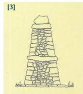
This profile shows the construction of a dry-stone wall. Two faces of wide flat stones are carefully placed with space between them, packed with smaller stones but not too tightly, as this is a favourite hiding place for much Cotswold wildlife. Larger stones are then placed on edge along the top, forming a strong wall capable of withstanding very high winds. The sides of the wall slope inwards towards the top—this 'batter' giving the wall more strength.
