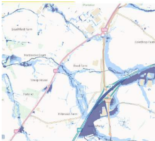
Figure 9. Extent of Surface Water Flooding
