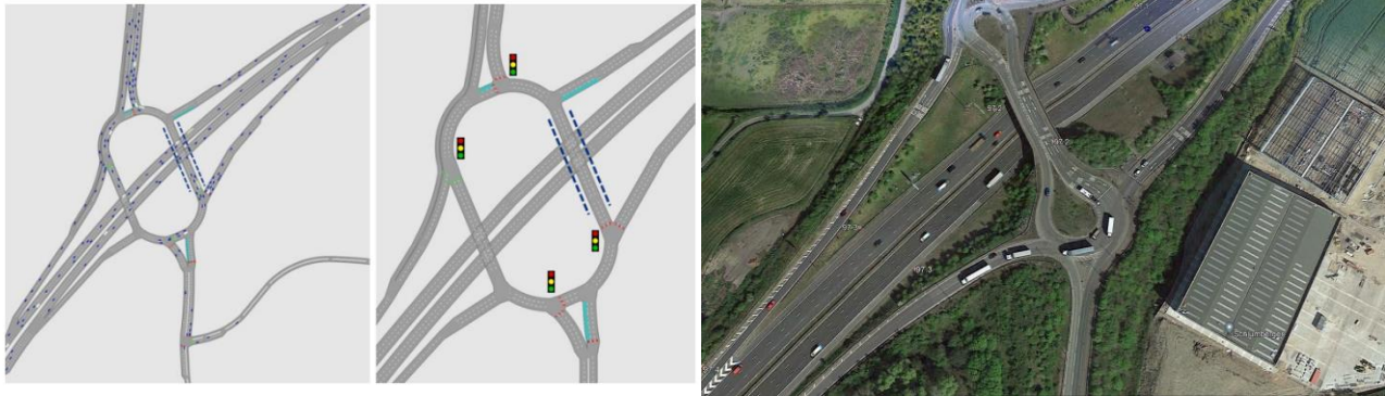
Figure 4-2 Option 4, upgrade of J12 to a Gyratory Junction
