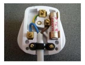
**Step 1:** Remove the plug cover either by unscrewing it, or sliding the cover off the plug base, which is the main part with prongs for plugging into an outlet.
